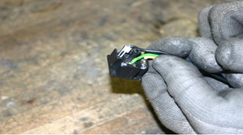
Figure 4: Terminal Block example with loose connector (black wire)
