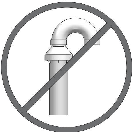
Figure 5-5 Do Not Install U-Bend to Rain Cap
